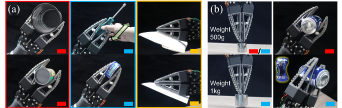
Fig. 3. Multi-mode grasping enabled by stiffness modulation and switchable adhesion. (a) Three grasping modes: compliant grasp (red) for conformal contact, stiff grasp (blue) for load-bearing holding and disturbance rejection (the screwdriver remains secured under manual perturbation), and adhesive grasp (orange) for attachment-assisted grasping. (b) Stiffness-dependent trade-offs: the stiff mode lifts a 1kg weight by fingertip pinch, whereas the compliant mode cannot; conversely, the compliant mode grasps an empty aluminum can without visible deformation, while the stiff mode crushes it.
