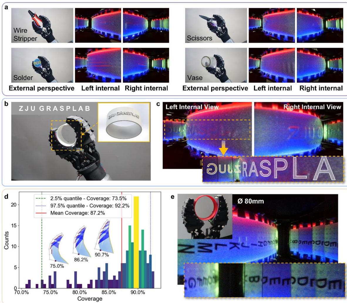
258 **a** Raw internal images captured while gripping various objects. **b** 3D-printed text ring. **c** Internal raw image
